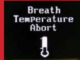
The breath temperature abort occurs when the breath blown into the device is inconsistent with the normal temperature of human breath. This may be due to you drinking an iced drink or exercising in the cold just before a test. If so, just wait a few minutes and try again.
